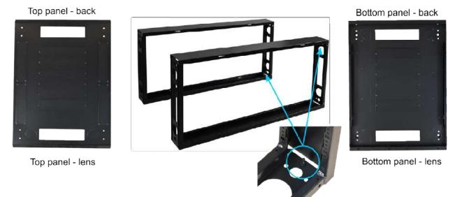
Mount the top plate and bottom plate to the left and right frames of the RACK cabinet, respectively. Use M8x12 Head Cap Screws with M8 nuts (16pcs). Screw the cabinet **wheels** and **legs** to the bottom plate of the cabinet.
